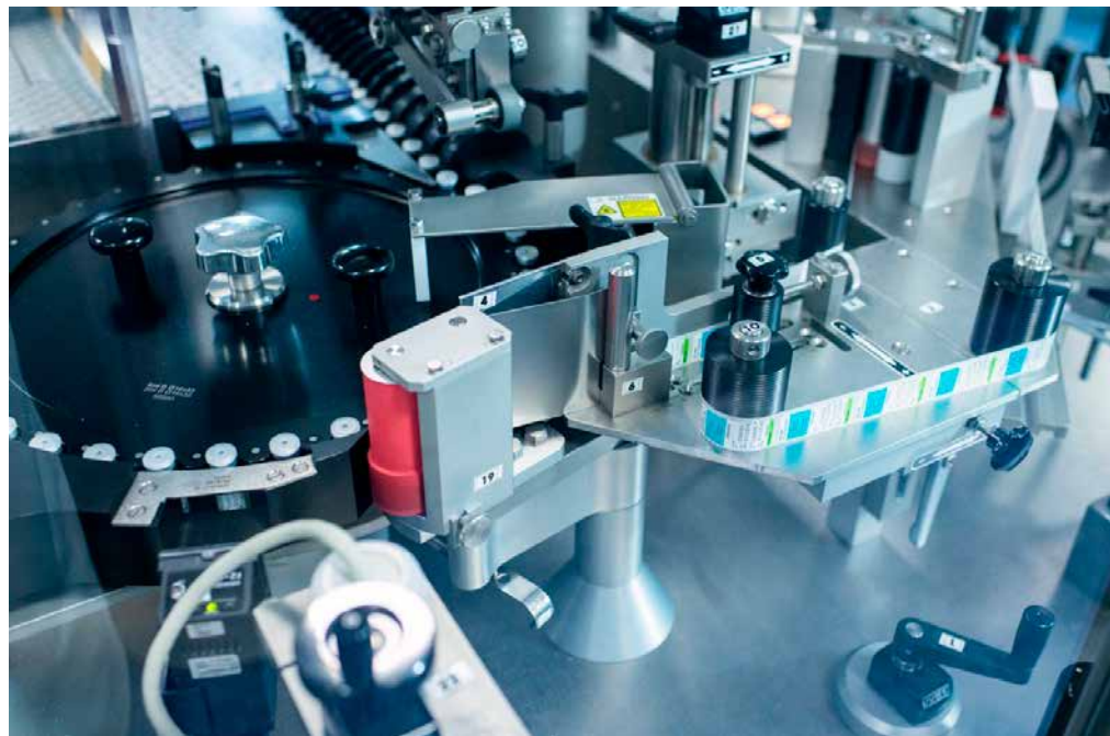
A vial labelling machine used for packaging of various finished products at Biovac's facility in Cape Town.
